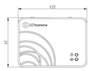
The APsystems Communicator, our state-of-the-art Energy Communication Unit (ECU-R), is the information gateway for our APsystems inverters. It collects and transfers module performance data in real time, giving you comprehensive monitoring and control over each individual module, optimizing the performance of your solar array.
